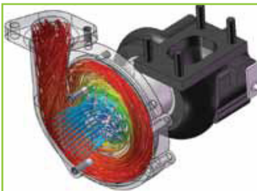
FloEFD can show the visual results of 'Flow Field' analysis in several formats; shown here as stream lines that can be tracked from point of origin to point of exit
